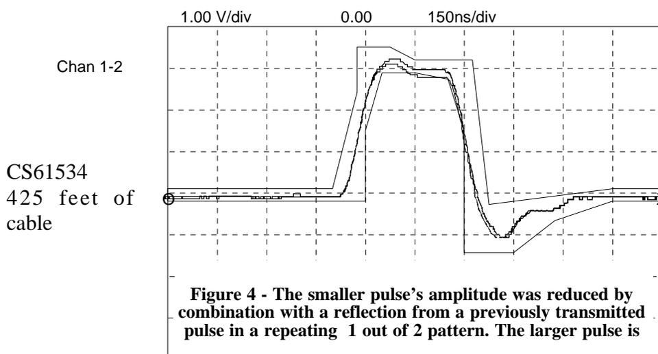
reflections. In order to avoid reflections in a transmission line, impedance mismatches should be avoided, and the line should be terminated with a load that is equal to the characteristic impedance of the line. Proper terminations are every bit as important when measuring pulses in the lab as they are in connecting up the network.
