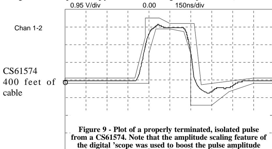
**Figure 9 - Plot of a properly terminated, isolated pulse from a CS61574. Note that the amplitude scaling feature of the digital 'scope was used to boost the pulse amplitude**
